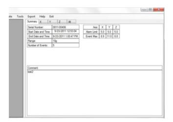
The table on the right hand side provides details of the alarm threshold setting per axis and the number of events seen per axis.
