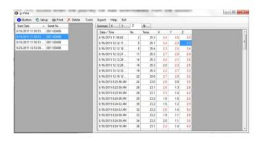
When any Event value exceeds the impact threshold limit entered in Setup for the journey they are shown in red; and where values have reached or exceeded the g-View units recording limits, defined by the products range, the Event data is underlined as well as in red.
