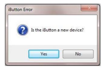
Click **Yes**. The iButton family will now be detected, but as this is a new device, the Function will show as Invalid - this is normal. Again click on the **Program** tab, to show the programming options for the iButton device.
