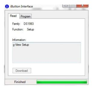
Remove the Setup iButton from the adaptor; and replace it with a Download iButton, if this is also a new device then the new device message will be displayed, again click **Yes**.
