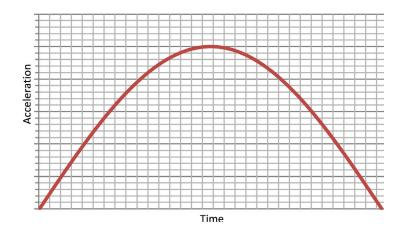
ShockWatch impact indicator shock response curves are based on a half-sine shock pulse (shown above). A time, acceleration point on the half-sine curve can be correlated to the same point on the impact indicator activation response curves.
